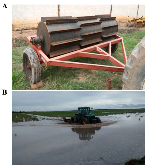
Fig. 4. Knife-roller (A) and management of irrigated rice straw with a knife-roller (B). Source: Alberto Baêta dos Santos.
